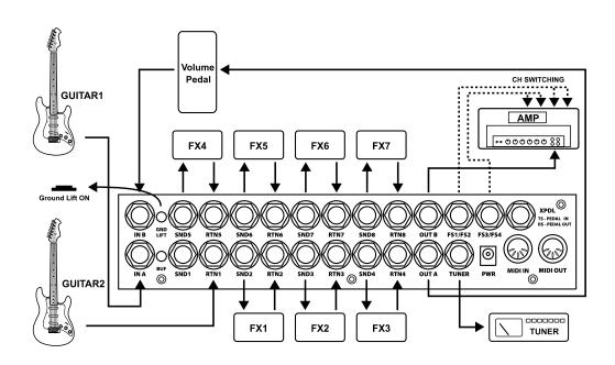
\* System with output switchable to either of two amplifiers being used
