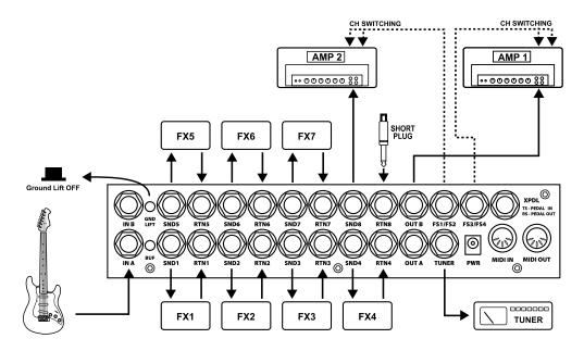
\* System with output switchable to either or both of two amplifiers being used
